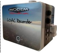
LCAC is the state of the art analyser consisting of an aerosol particle counter providing size distribution and typology while offering a high level of sensitivity. This new, unique and versatile aerosol monitoring instrument does not needs any lense. It uses a laser beam and measurements are conducted at two scattering angles, of 12° and 60°.
