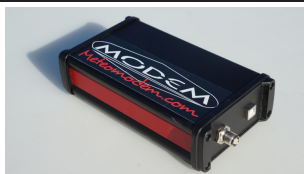
Pilot Ground Receiver
