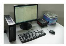
Main function of the Rio upper-air radiosounding system consists in collecting P,T,U, and wind data measured and transmitted from a Meteomodem radiosonde by radio telemetry.
