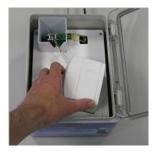
**Groundcheck** for Radiosonde calibration before launch
